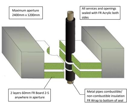
Smoke-safe (<0.1m<sup>3</sup>/h smoke leakage at 200Pa)
